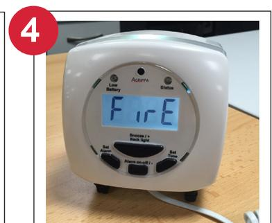
4 High intensity LEDs will flash and the screen will display "FIRE."
